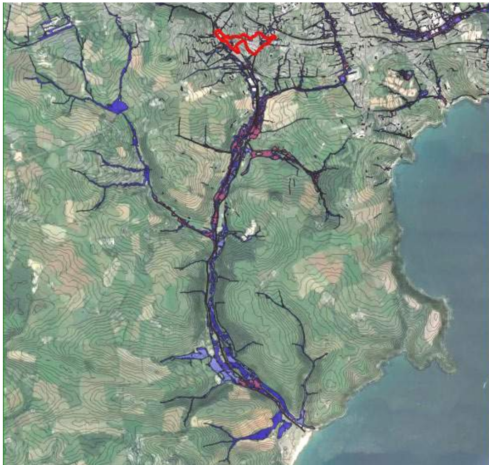
Image 3.1. The Environment Agency fluvial model overlay, with Site Contours overlaid by the author, depicts the probability of flooding in St Austell's River using historical data (High (Magenta), Medium (Dark Blue), Low Risk (Light Blue))
