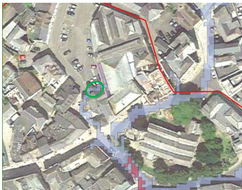
Map showing the areas at risk of surface water flooding overlaid on Google Maps. The rain garden location (Green Circle) at the lower south end of Market House public realm would capture stormwater at its source and prevent flooding further downhill.
